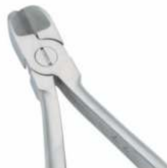
SI5008 Hard wire cutter, easily cuts any size arch wire or pin. The inserted tips ensure precision cutting and perfect tip alignment. Minimum Cutting Capacity: .012"(.30mm) Maximum Cutting Capacity: arch wires up to .021"x.025"(.55mmx.64mm)
