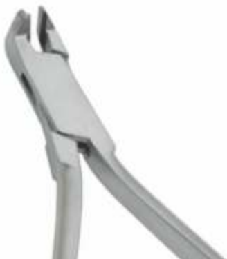
SI5002 1-Distal End Cutter This instrument cut wires close to the buccal tube and safely holds the distal end. The tungsten Carbide insert ensure precision cutting, long wear and unsurpassed cutting performances. Maximum Cutting Capacity. arch wires up to .021"x.025"(.55mx.64mm)
