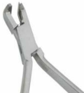
SI5003 1-Distal End Cutter Flush Cut with Safety Hold This instrument cut wires close to the buccal tube and safely holds the distal end. The tungsten Carbide insert ensure precision cutting, long wear and unsurpassed cutting performances. Maximum Cutting Capacity. arch wires up to .021"x.025"(.55mx.64mm)
