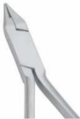
SI5040 Slim Bird Beak Plier This popular loop forming and bending plier has inserted tips that provide excellent wear. The precise round and square tips bend arch wires from .012" to .020" (.30mm-.51mm) Wire bending capacity: .020" (.51mm) Also Available in TC-Tip
